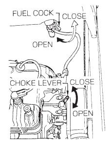
Figure 5. Fuel Cock and Choke Lever
